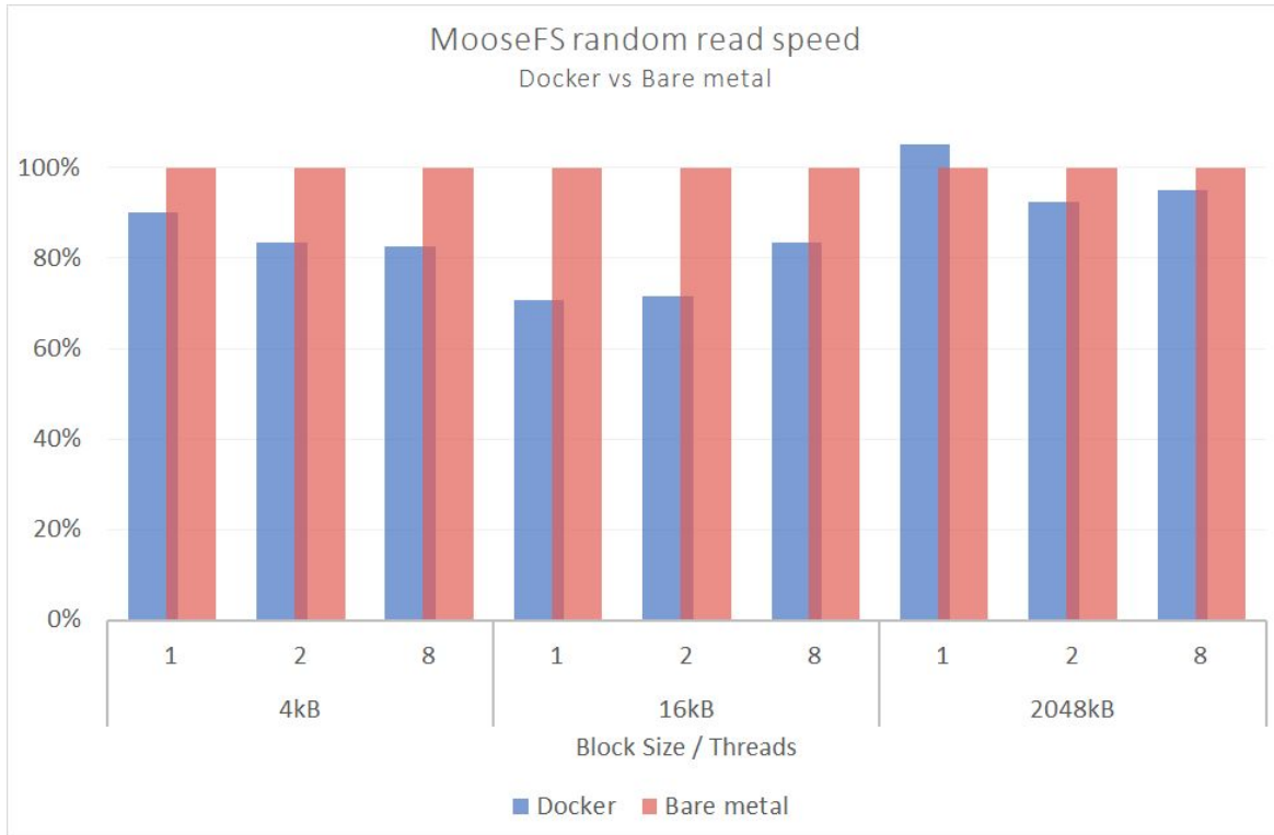
Figure 4: Random read speed test results using 1, 2, 8 threads for each 4 kB, 16 kB, 2048 kB Block Size
