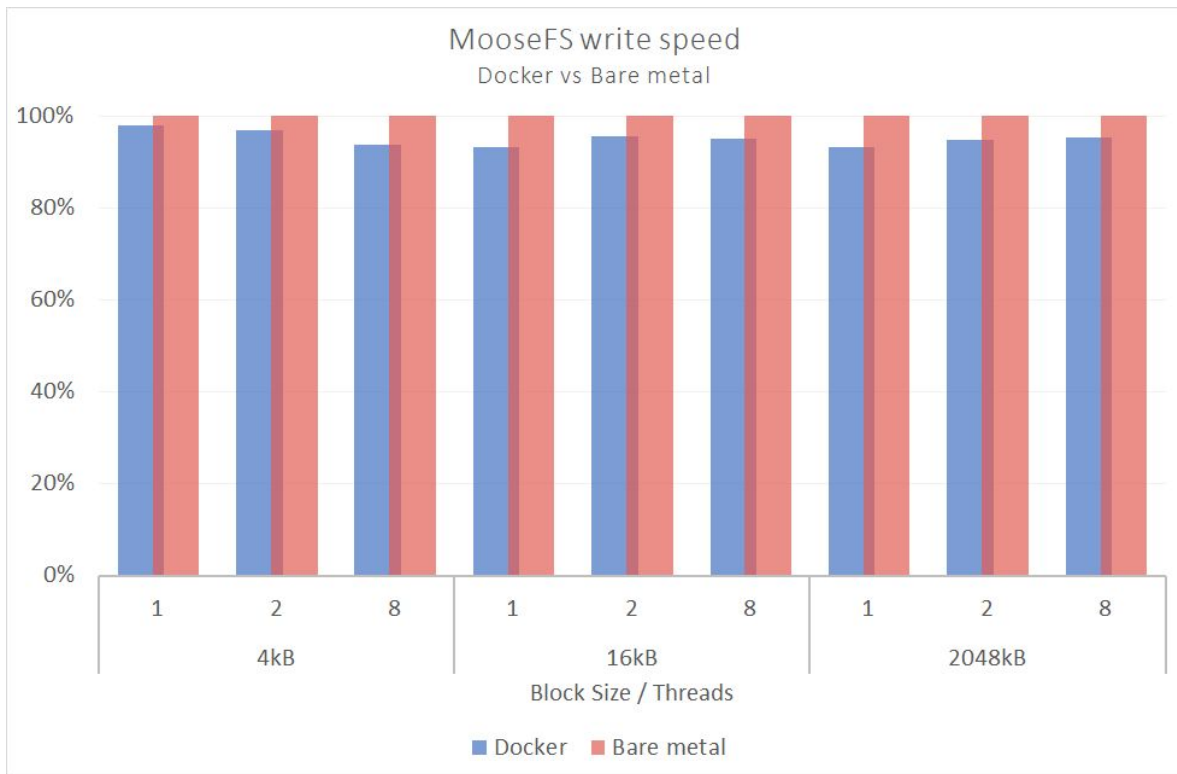
Figure 3: Write speed test results using 1, 2, 8 threads for each 4 kB, 16 kB, 2048 kB Block Size
