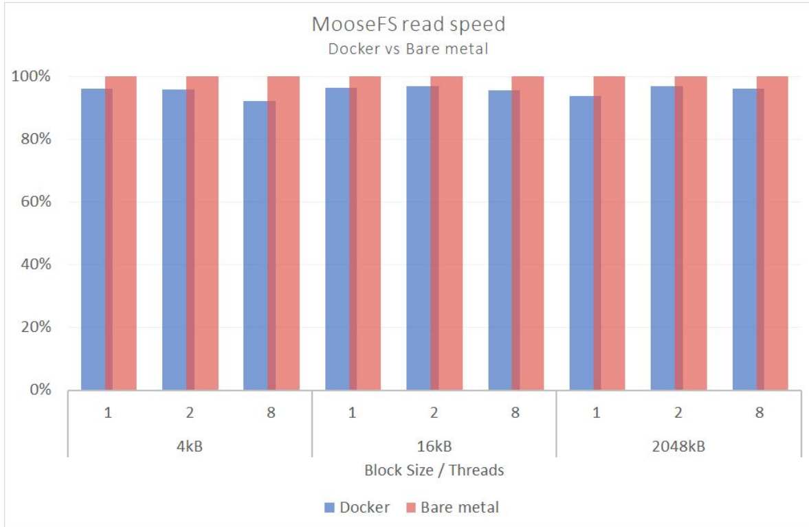
Figure 2: Read speed test results using 1, 2, 8 threads for each 4 kB, 16 kB, 2048 kB Block Size
